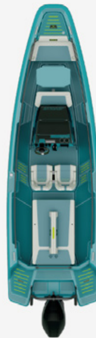
Multi storage compartment w. optional cushions, forward facing console seat, removable cockpit table, front deck seat
