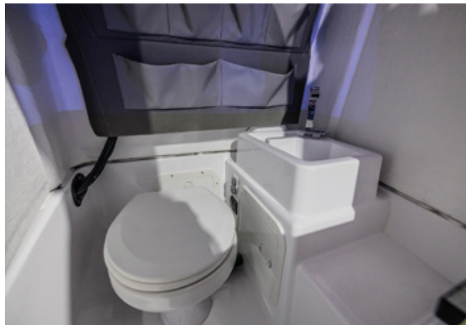
Toilet, electric fresh water flush, 20 l septic tank
