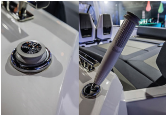
Fresh water system 40l+ shower on aft deck
